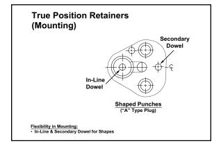
The secondary dowel is used to radially orient a shaped punch. This dowel hole is precision ground on the same center line as the punch and ball holes to guarantee proper radial orientation.
